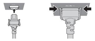
1) Check the shapes of the <AC IN> terminal on the back of the projector body and the power cord connector and insert the plug completely in the correct direction (until you hear the side tabs click in place).
