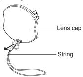
2) Thread the other side (the side with larger ring) of the string through the hole at the bottom of the projector and fasten it.
