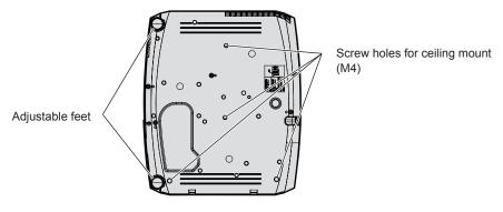
Positions of screw holes for ceiling mount and adjustable feet
